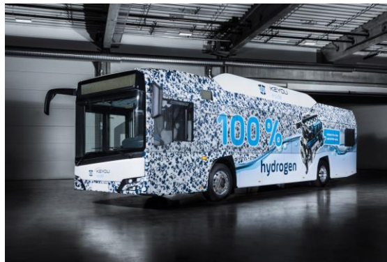
A bus powered by hydrogen with a it's conventional engine, Keyou is the company behind it (Image 8)
