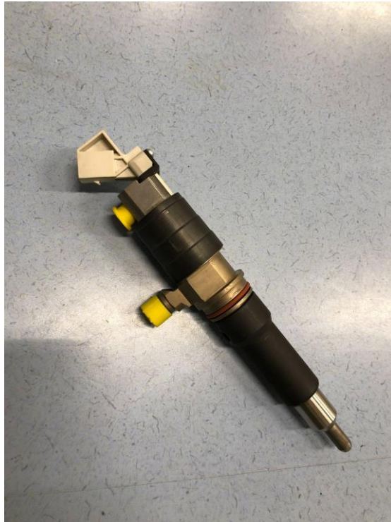
Here is one example described, this dual injector is developed by the company West port. (Image 23)
