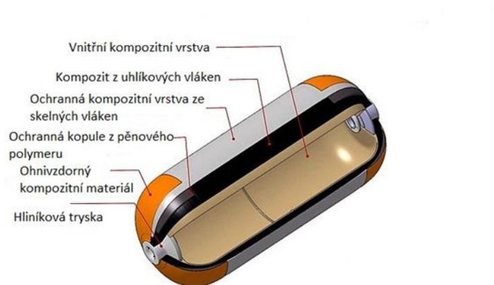
Fig 5: Cross-section of hydrogen cylinder
