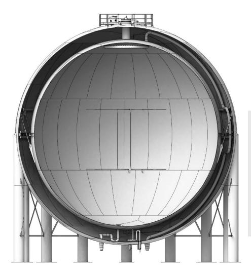
40,000 m<sup>3</sup> liquid hydrogen storage Vessel
