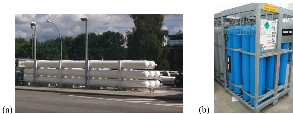
Figure 4. The examples of hydrogen storage vessels common for stationary applications: (a) fixed bundle of cylinders, (b) a basket of cylinders.
